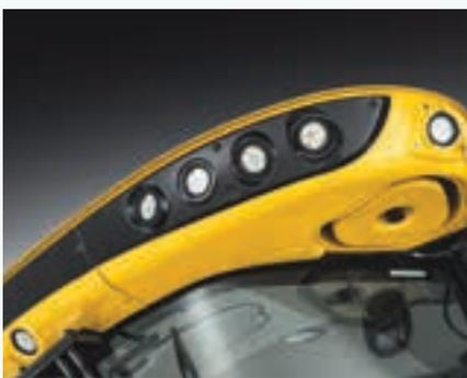
The FR lighting package offers up to 20 work lights including 17 LED lights. 11 LED lights have been precision placed in the roof to ensure the perfect spread of light.
