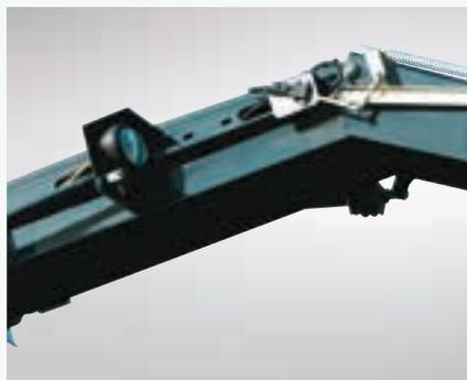
Six working lights have been placed in key working areas, including the spout, service deck and on the bumper to enhance foraging accuracy when working in low light conditions.
