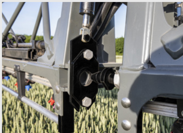
A stop-and-lock system avoids slack between the boom sections, which are folded and unfolded smoothly with SoftOpen/SoftClose.
