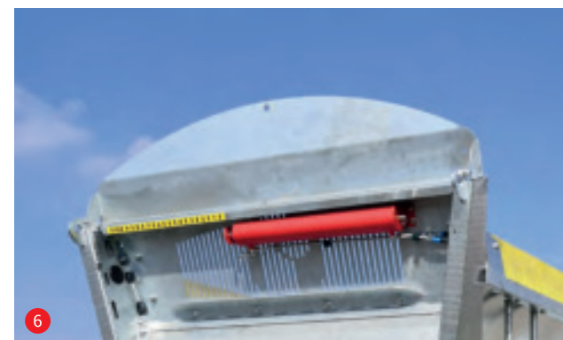
5 | Mechanical guillotine door opening indicator
