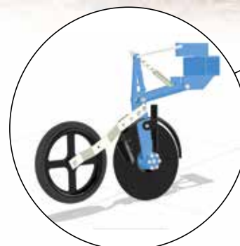
Double disc couler For an even germination rate
